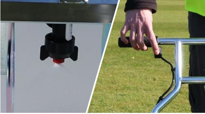
**9. Turn the machine off as the paint starts to spray out the nozzle.**
